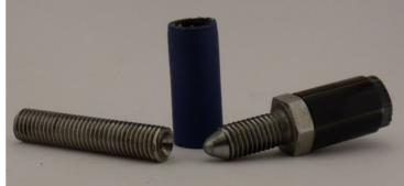
The flexi coupler consists of a short length of thread with a dimple in one end. This mates up with a rounded point on a bolt. They are held securely together with a tight fitting piece of rubber hose. A sacrificial piece of wood or plastic is glued to the head of the bolt. This gets glued to the blank.
