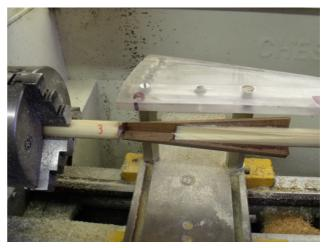
The result of cutting deeper than the middle of the blank can be seen in the above picture and the reason should also now
