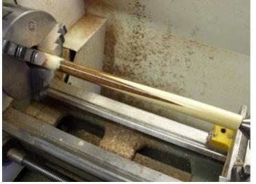
In this pic, I have removed the ramp and turned down the blank. Ready to make into a pen.
